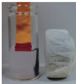
Figure 3. The behavior of Co@SiO 2 to a magnet (right) after immersion in 1 M HCl for 1 year. Particles in the sample bottle are gathering near the magnet (left). The photograph also shows that the color of the pH indicator paper turned from yellow to red in the acid solution.
